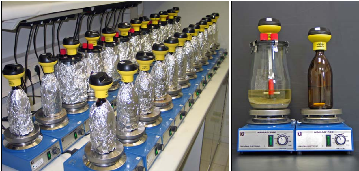
Fig. 3: Left: Experimental setup in the test with ivermectin and atenolol. Right: Newly developed water-sediment system and standard water-only system
